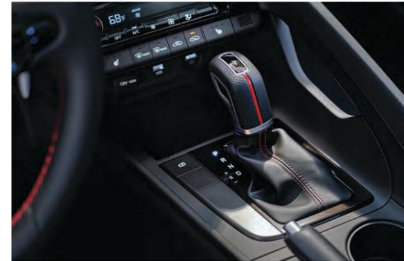
N Line: 7-speed Dual Clutch Transmission
