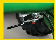
Convenient single-point hydraulic connections save time while eliminating connection error with virtually no oil loss. Plus, electrical connections are integrated in the single-point connection.
