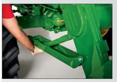
Parking stands and pins are integrated on the loader – no loose parts, no tools needed.
