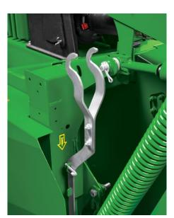
Change knives in minutes, using only this quick change tool, which attaches to the back of the Mower-Conditioner for easy access.
