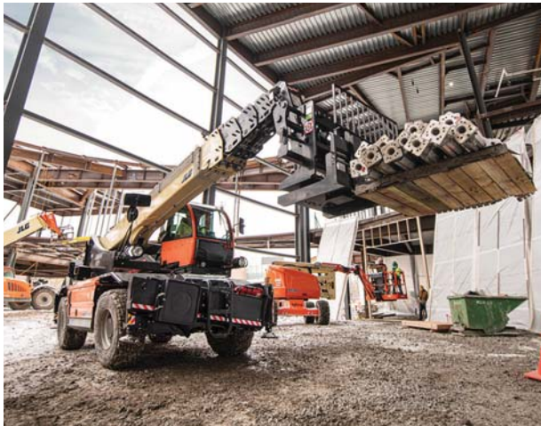
JLG is launching a new group of rotating model telehandlers offering users capacities from 11,000 to 13,000 pounds and reaching up to 97 feet. Photo by JLG
