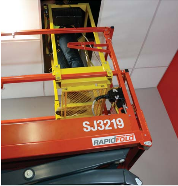
Operators can step up almost 19 inches into the XStep, close the top rail and safely gain extra jobsite access.
