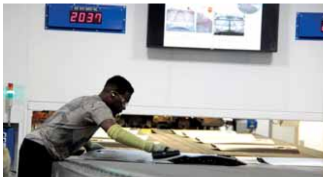
A quality check is performed on a freshly stamped door at FCA's Warren Stamping Plant, Michigan
