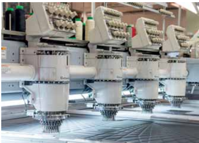
New quilting machines at Gaydon, developed alongside a Japanese supplier, allow for larger hides to be fed through
