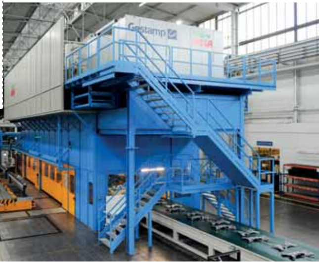
The 37-metre long, 1,350-tonne servo press at Gestamp Bielefeld
