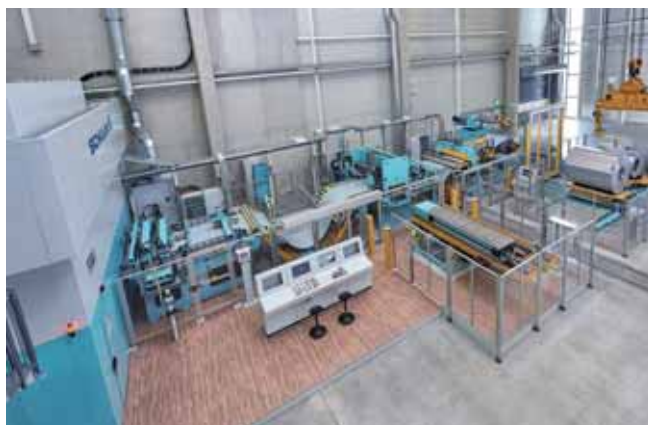
Daimler has commissioned two laser blanking lines using Schuler technology at its plant in Kuppenheim, Germany
